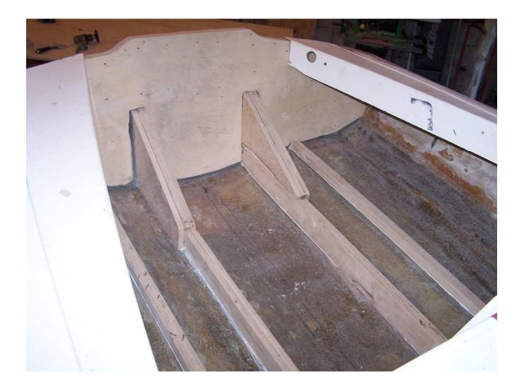
Clean up adhesive on edges, and dress rough edges on exposed SS fasteners. (Knee Braces) and remove screws that went into the temporary blocks. (and remove blocks.) Adhesive around edge will hold the curve once cured even with the blocks removed.
