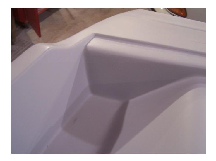
Ready for a final sand and paint. Application of 3M Dry Guide Coat which is a black carbon powder that sticks to all surfaces. Final sanded with 400g abrasive on a DA sander. Dry Guide Coat that remains during this process may indicate a problem. (pinhole, scratch, etc.) Sand until gone, and fix defects as necessary.
