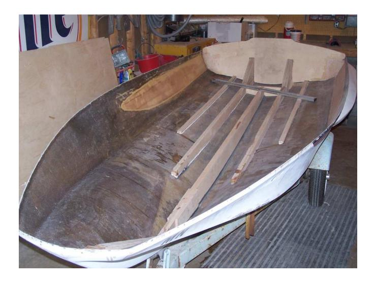
For resin and matting to lay down properly, all 90° angles must be radiused with a fillet putty or body filler
