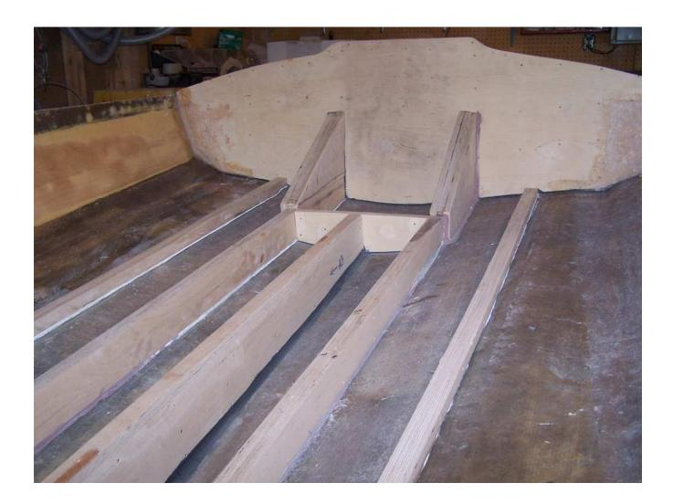
Close up view of harsh angle. Too much for matting to lay down with out having voids in the laminate.
