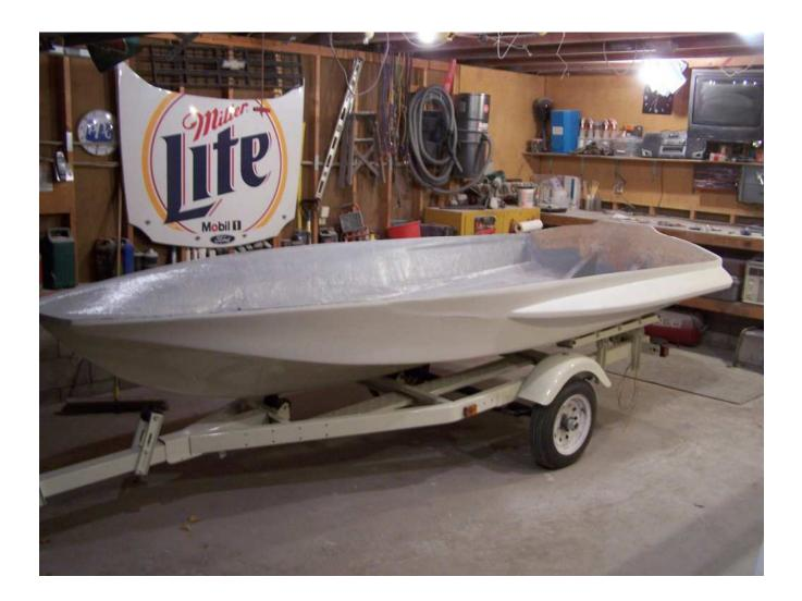
Back to the deck which now has completed body work and has been primed, blocked and reprimed.
