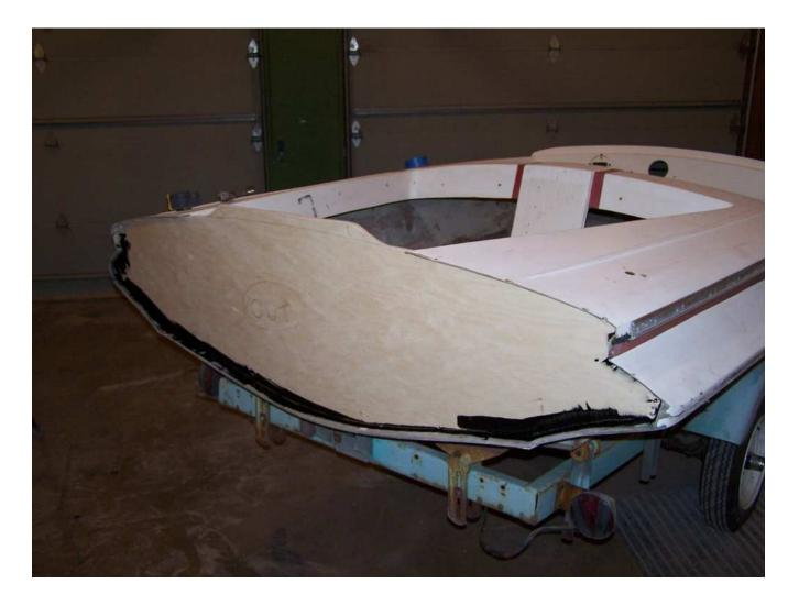
Build Knee Braces if desired after the first layer of transom is secure. This way, they can be mechanically secured to the transom prior to the addition of layers 2 and 3 of transom wood. Ensure they are not too high and will not interfere with the splashwell.
