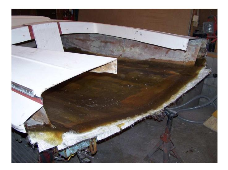
Glass work is trimmed and sanded. This hull had no stringers, and no patterns were available. I created them from scratch using thin strips of luan board to find the correct shape. (easier to work with.)
