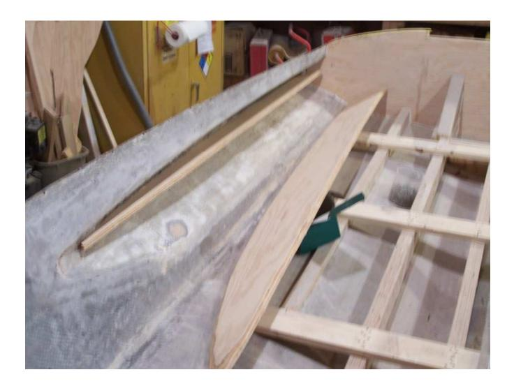
Once attached, the outer trim screws are again removed and the complete assembly can be taken out.
