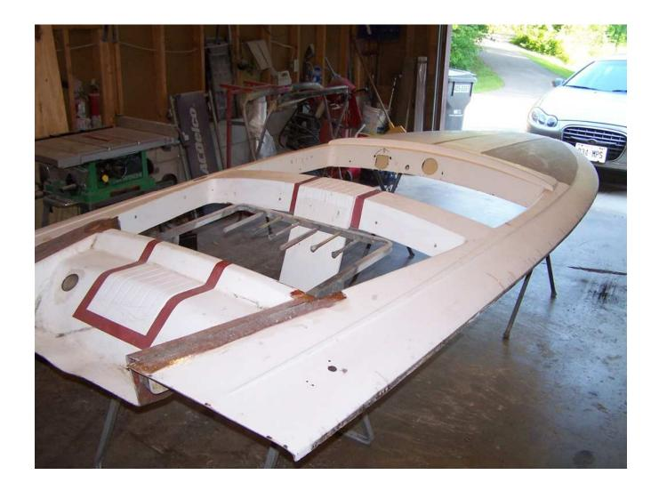
Remove all rotten wood. I used a 2.5" cold chisel... sharpened to a fine edge and tapped along the FRP and wood mating surface. This cleanly removed the rotten wood and left a relatively smooth surface.
