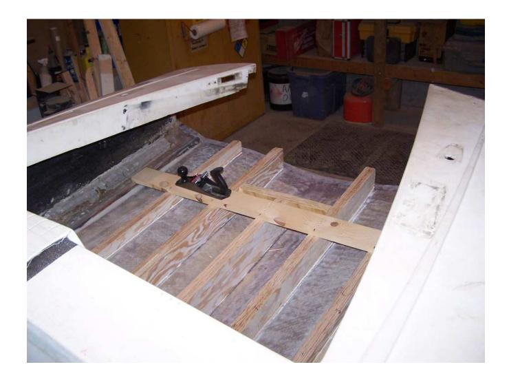
Use saved FRP cutout and trace onto 1/2 " plywood. Make 3 of these to achieve the factory 1.5" thickness. Trying to bend ¾" wood is too challenging. Use weight to "bow" each pre-cut piece of transom wood. Hose down with water occasionally over a few days in this position to retain the shape. I had over 100lbs on this piece for about 36 hours. It was perfect!
