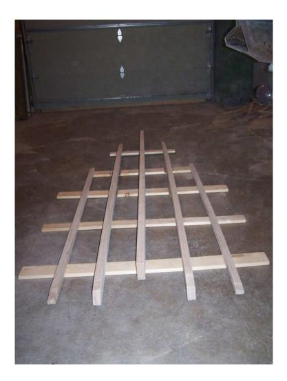
Assembled skeleton. Each stringer is double stacked. 1.5" thick wide each. They are laminated together with 3M 05200 Marine adhesive, and screwed together with stainless steel deck screws.
