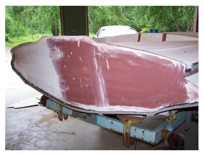
Use ¾" SS deck fasteners to solidly screw the next layer into place, and backfill edges with 05200 adhesive. Repeat this process for layer 3 and allow to dry thoroughly. Finished product should look like this! Be mindfull to not place screws where you may drill later... (Engine mounting, ski / tow hooks etc.)
