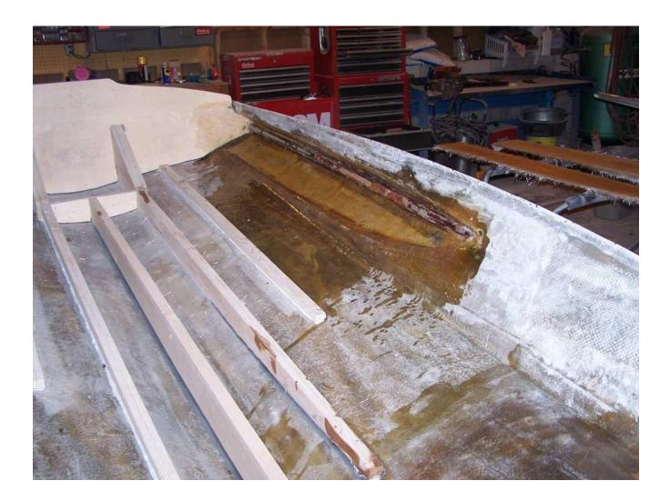
Made new sponson support wood. Fastened it into place from the outside to allow attachment of the inner panel on the boat.
