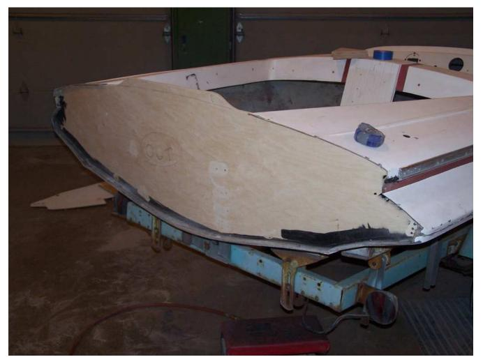
Notice the proper curve of the transom and the 1.5" setback of the first of 3 layers. Layer 3 will be flush.
