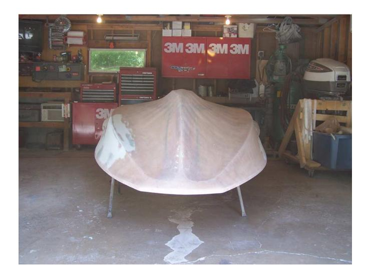
Two good coats of vinyl-ester primer surfacer is applied to fill in imperfections and seal the hull. (vinyl-esters are suitable for below the water line.) It is blocked smooth and straight with 180 grit abrasive, and reprimed with two more coats. Final sanded using a DA and 400g abrasive.
