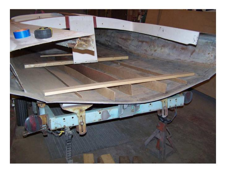
I then transferred those patterns to ¾" plywood, double stacked to make SOLID framework for this little boat.
