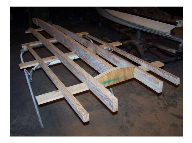
Install skeleton and trace with a sharpie. Remove skeleton and apply 3M 05200 Adhesive to hull inside the sharpie markings. Reinstall and ensure stringer assy is 1.5" forward of the stern to allow room for the transom.
