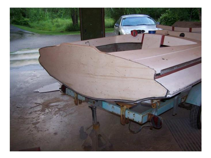
Identify position for splash well. (I am glassing it in permanently for improved strength and more of a fast-back look.)
