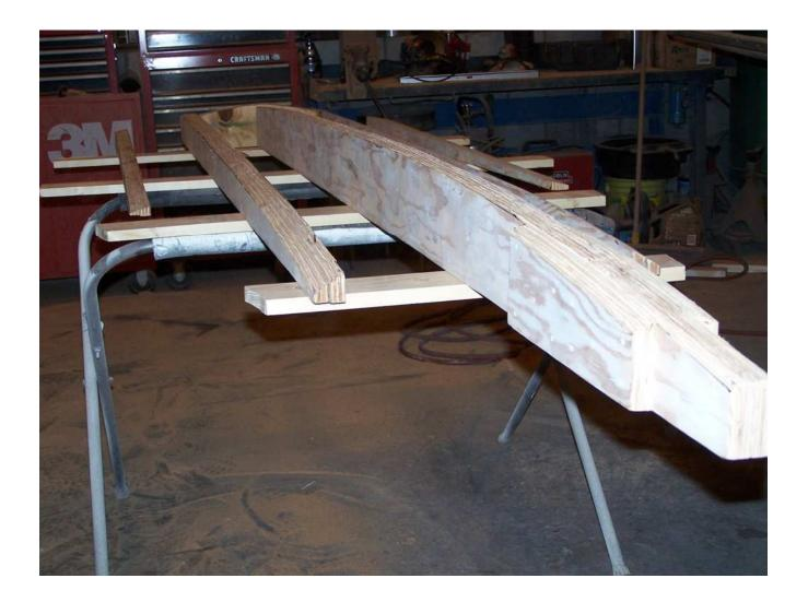
My favorite wood to work with so far for was baltic birch. It is a good hardwood, and is assembled with outdoor adhesive. The layers are thin and tight, and there are almost no voids in the laminates.
