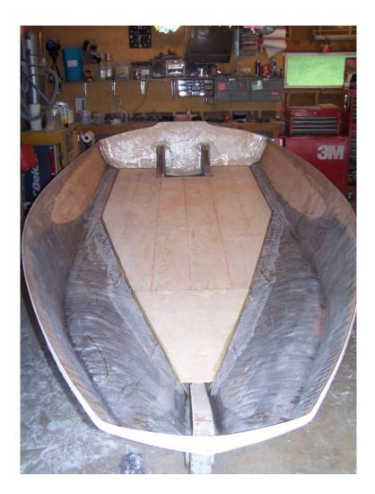
Rough and square edges smoothed off with a grinder, followed by a fiberglass strand reinforced putty applied to the floor to hull joint.
