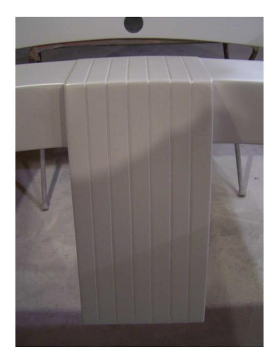
Deck reinstalled and permanently bonded and bolted to hull for rigidity. (Note, I did not use the factory type molding. It was junk and not replaceable. This method is more work, but stronger!) ¼" x 20 machine screws, countersunk with washers and lock nuts. 4" on center all the way around.
