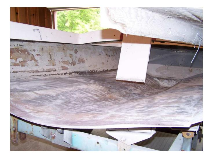
Cut all matting in advance to make it easier while applying resin. (Different hull than previous pictures.)
