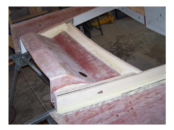
Woodwork around the bow. (note, I laminated the entire surface of the deck on the inside after removed old woodwork, and before installing new wood. I wanted a SOLID deck, not the flimsy factory deck.
