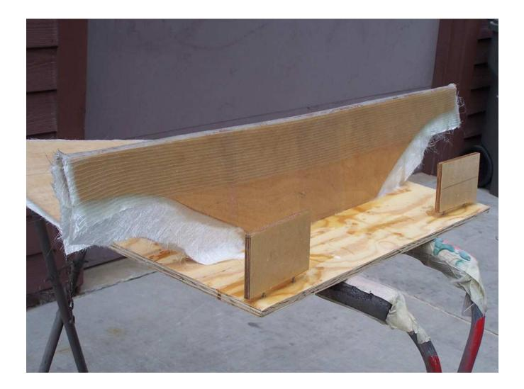
05200 adhesive applied to the top of all stringers. Floor installed and screwed into place with 1.25" SS deck screws.
