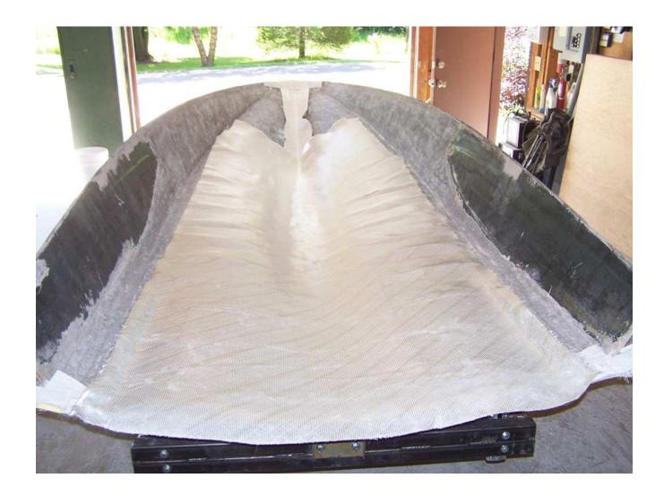
Laminated with polyester resin. The first of 18 gallons used on this project. At least now it won't break as I crawl around in there!
