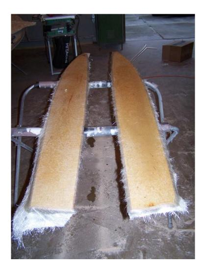
Cracks repaired from the inside with matting and resin. Will fix from the outside also for extra strength.
