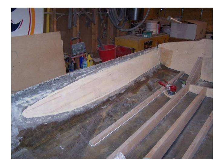
Because bigger is better, I replaced the tiny rotten eyelet wood with a piece that connected down to the center stringer. Wicked Strong!
