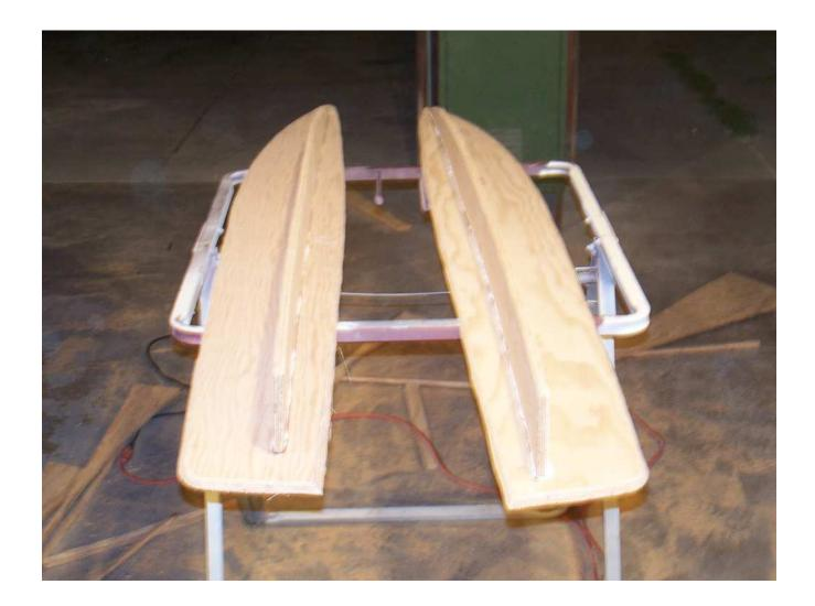
Installed. Set in 05200 adhesive. Held in place to dry with trim screws along length of sponson. (factory holes.)
